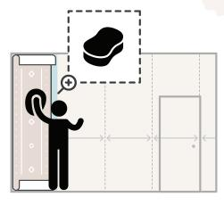
To get rid of air pockets, use a clean roller, sponge or brush, taking care not to squeeze out the paste between the joins and ensure the paste does not get onto the smoothing roller or sponge.
