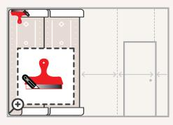
Use a sharp snap off blade knife. Push the paper into the ceiling line and skirting. Replace the blade often, as a dull blade can easily tear the wallpaper.
