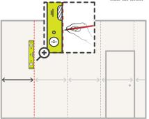
Using the header, measure this amount out from the corner (in the direction you are going) minus half an inch.
