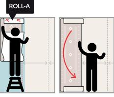
Attach the top of the length to the wall at the preferred height and in the correct position before letting go of the rest.
