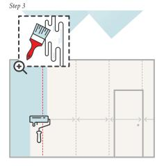
Our wallpapers are made using on a non-woven base. That means you apply the adhesive directly to the wall. Start by pasting an area sufficient enough to cover just over one drop width at a time. Use a paintbrush to cut-in around the areas too tight for the roller. (Such as at the ceiling line, corners, and along baseboards and trim).
