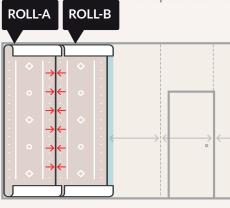
Butt join the Roll A length and the Roll B length together, matching up the edges. Ensure that the lengths are properly positioned, that the pattern is matching and there is no surface visible at the joints. It is important that adhesive be applied right out to the edges to ensure the lengths adhere to the wall properly.
